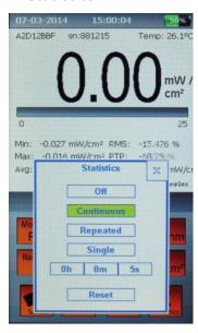
The Statistics key opens the corresponding window . Four processing options are available:
