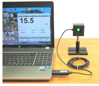
The PC-Plug sensors have been primarily developed for applications that need a power measurement station on board of machines, like in laser marking, cutting, welding, micro-machining; these instruments are also the perfect monitoring tool for other industrial applications such as laser burn-in or long-term reliability testing.
