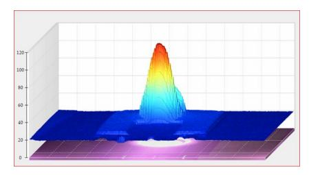
Mod. W-12K-D55-SHC-USB: Thermal images of the absorbing surface at 10 KW- Max. Temperature on the coating is 113 °C (IPG fiber laser YLS 10000)
