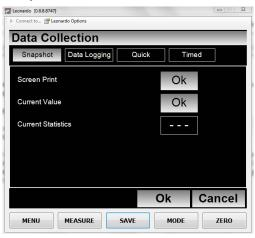
This mode allows to save the screen content, and/or the last value of the measured function and/or the relative statistics .
