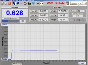
This family of detectors is used for accurate, yet once in a while readings and whenever simple power checks instead of long term measurements are needed. In this configuration the operator only has to expose the head to the laser beam and, after the correct timing generated by the PC Link's internal firmware, the measurement is over. (There is no need to provide the time window to the laser shutter)
