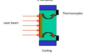
Light penetrates through a thin layer of optically absorbing refractory materials (10-40 $\mu$ m thick ) . Generated heat flows through the substrate toward the thermocouple array and the cooling system.
