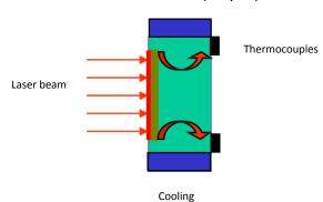
Light penetrates within the same thin layer of optically absorbing material, as previously shown. During the shorter laser pulse duration, the suddenly generated amount of heat cannot flow through the substrate. Major damages to absorbers may occur. Volume Absorbers offer far better performances.
