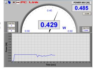
graph are pinned to the last power value acquired before the alarm.
