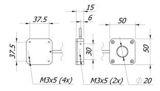
CSA-2-D12-BBF-USB /CSA-2-D12-BBF-RS CSA-2-D12-HPB-USB /CSA-2-D12-HPB-RS CSA-5-D12-BBF-USB /CSA-5-D12-BBF-RS
