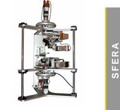
**OFF-AXIS TESTING OF SMALL LENSES** Full 360° coverage in  $\phi$ , ±35° in  $\theta$ Mobile phone camera lenses **Digital camera lenses** 7-axis motor movement with encoders • **Aspherical lenses** • Vis wavelength range (400nm-1060nm) 9 **On-line alignment of complex lenses** Full software for control and analysis × Zernike coefficients, WF, MTF etc. SMALL LENSES ----() **Full accessories**
