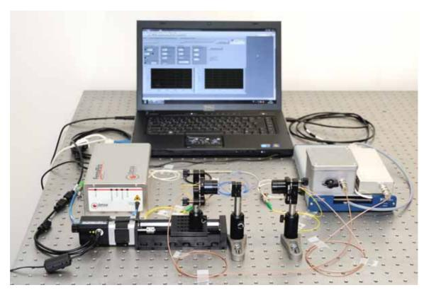
Fig. 1: Fiber-coupled THz time-domain spectrometer with THz focus
