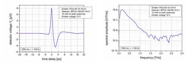
1560 nm fs laser with emitter PCA-40-10-10-1550-h-f and detector BPCA-100-05-10-1550-h-f
