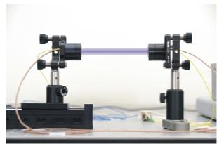
Fig. 3: figurative terahertz path - collimated option
