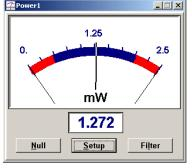
Display power with analog and digital displays.
