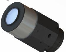
AngleMeter LA measures laser beam deviations with respect to housing (in mRad), by monitoring the beam angle in two orthogonal directions. The new instrument meets customer's requirements for a variety of optical testing, both for laboratory and production floor. Equipped with a large input aperture lens and a high-accuracy detection capability (provided by PSD type detectors), the system measures minute deviations in a relatively large field of view.
