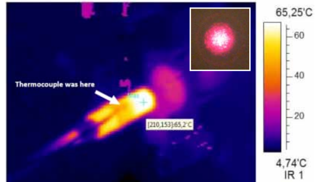
IR-image of common Fiber Cable assembled with mode stripper & radiator at the output end
