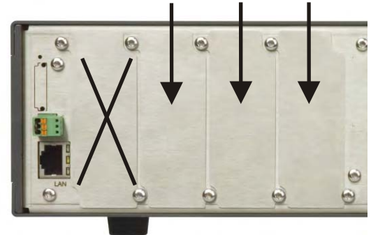
fig. 4 - 1 Positions for the INT MOD SIM.
