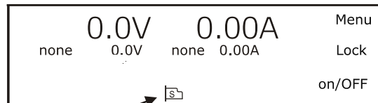
fig 3 -4 Position of the interface Slave icon in the unit display.
