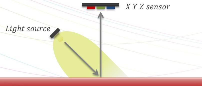
Fig 1 45/0 degree measurement principle.
