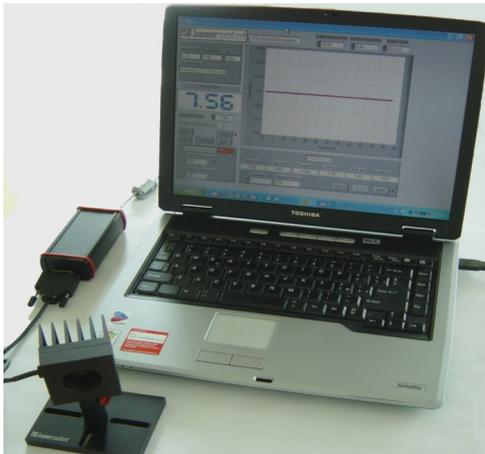
LaserPoint's **PC-Link** is a smart head to USB interface that converts any PC or laptop into a powerful instrument which measures, analyses and records power and energy from any of LaserPoint detector heads.
