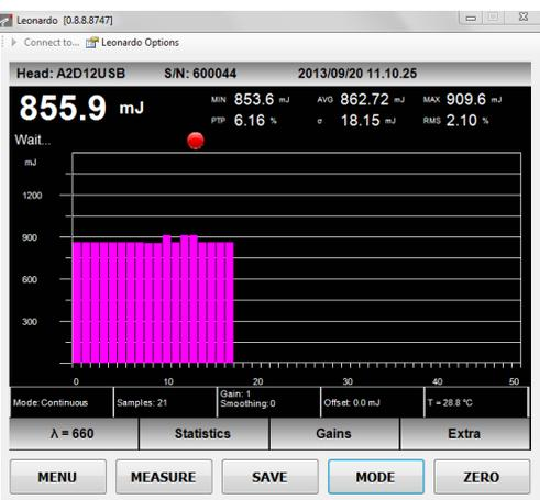
The energy display mode screen is a histogram-like graph where the energy of each laser pulse is represented as a vertical bar and the last measured energy value is also digitally shown . The statistical information about the measured data is shown in the upper part of the display.
