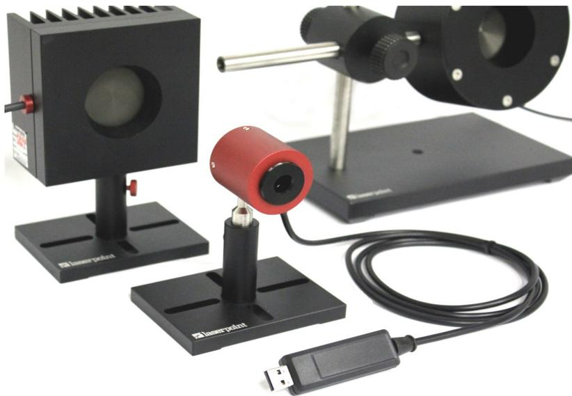
laser power measurement is subject to the same process. Traditionally the complete measurement set is made of a detector head connected to separate electronic unit to display results: Laser Point has developed a series of laser power measurement instruments introducing new microelectronics circuitry that has reduced the complete electronics to the size of a USB 2.0 or RS-232 plug.
