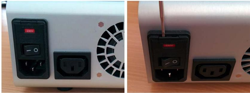
**Figure K.2:** To change fuse or voltage, open the fuse cartridge cover with a screwdriver inserted into a small slot at the top of the cover, just above the red voltage indicator.
