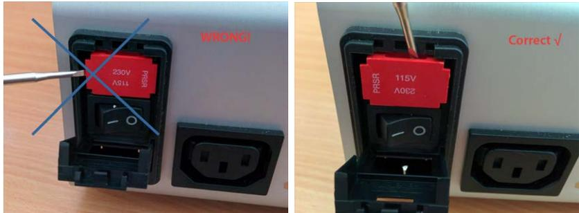
**Figure K.3:** To extract the fuse cartridge, insert a screwdriver into a recess at the *top* of the cartridge.
