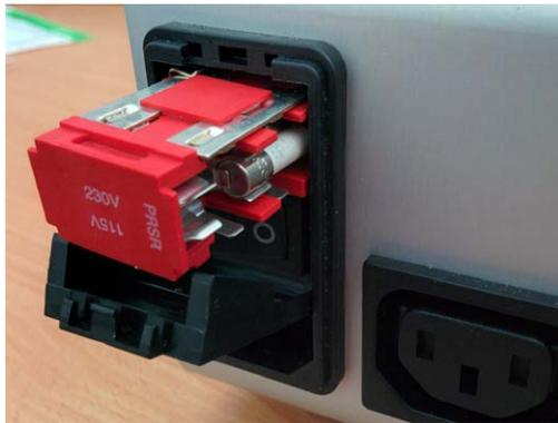
**Figure K.1:** Fuse cartridge, showing fuse placement for operation at 230Vac.
