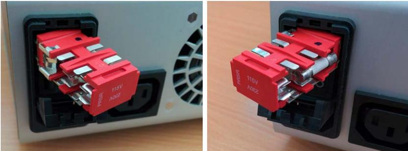
Figure K.5: Bridge (left) and fuse (right) for 115 V.
