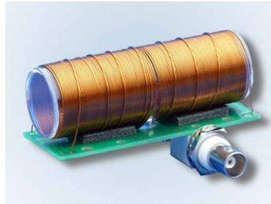
**Figure D.1:** Vapour cell, Zeeman coil, and primary excitation coil, mounted on PCB (available from MOGLabs).
