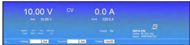
fig. 3 - 4, The front console of the web interface for setting of the input and monitoring various parameters.
