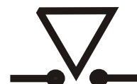
fig. 6 - 11 The Interlock symbol will be visible in the display when the link is interrupted.
