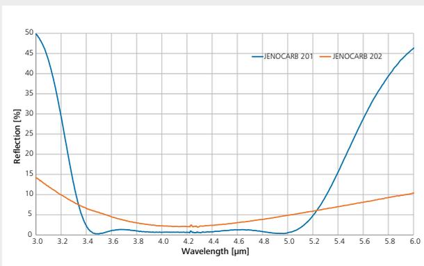
DLC and Hybrid-DLC for 3.0 - 5.0 µm on Si
