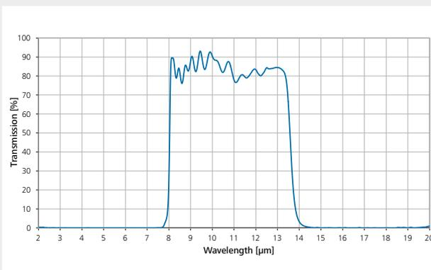
Bandpass Filter 8.0 - 14.0  $\mu\text{m}$  on Si
