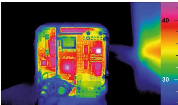
Electronics – sample thermogram, 1024 x 768 pixel thermogram recorded with IR-TCM HD
