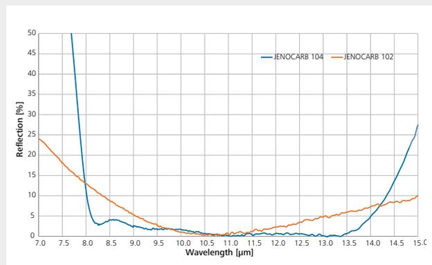
DLC and Hybrid-DLC for 8.0 - 12.0 µm on Ge
