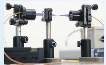
setup with one collimating and one focusing silicon lens
