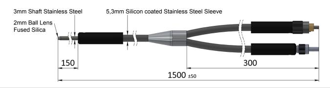
1x 9 Fiber bundle Dielectric filters for excitation and detection channels directly deposited on fiber ends.
