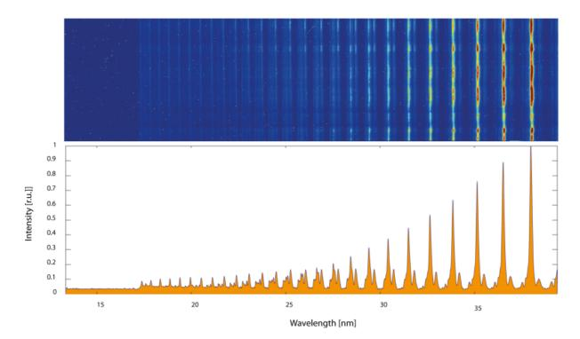
Sample measurement demonstrating the resolving power of the XUV spectrometer. The shown high harmonic spectrum is generated by the interaction of a single femtosecond laser pulse with a solid target and subsequent spectral filtering. The substructure inherent to the generation process is clearly resolved by the XUV spectrometer.
