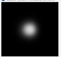
▲ 1.55 µm semiconductor laser beam image Interference fringe pattern may appear depending on laser beam wavelength and coherency.
