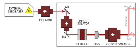
**Figure 4.1:** Configuration of MSA with internal seed laser, or MOA with external seed laser. For MSA, there are two internal input isolators between seed and amplifier. For MOA, there is usually one internal input isolator and one external.
