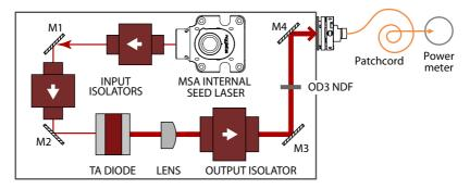
**Figure 5.2:** MSA showing addition of an OD3 neutral density filter between amplifier and fibre coupler to minimise risk of damage to fibre facet when operating at normal power and hence normal asigmatism and thermal lensing.
