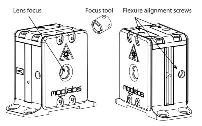
**Figure 4.2:** TA power block, showing location of flexure screws for adusting alignment of input and output lenses.
