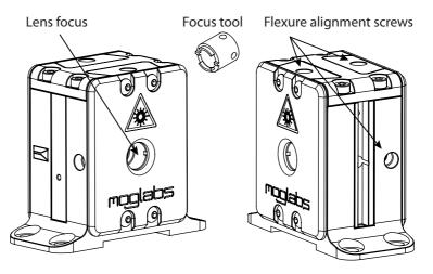
**Figure 3.2:** TA power block, showing location of flexure screws for adusting alignment of input and output lenses.
