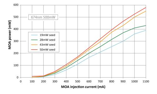
**Figure 3.4:** TA output against diode current, for several different injection seed laser powers (measured pre-isolator).
