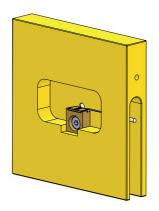
**Figure 6.1:** MGM-068 copper mount with C-mount TA diode seen from exit aperture side. Cathode pin, groove for cathode wire, and one registration pin hole are on right.
