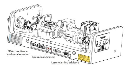
**Figure 2:** Schematic showing location of warning labels compliant with International Electrotechnical Commission standard IEC 60825-1:2007, and US FDA compliance label. Emission indicator for seed laser (left) and amplifier (right). Aperture label engraved on front and rear apertures; warning advisory label on right hand side, compliance label left hand side near exit aperture.
