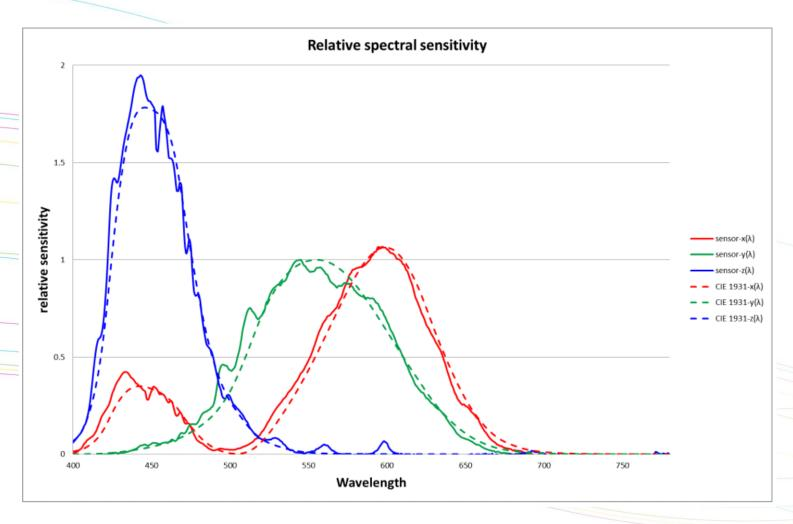
Fig 3 Spectral sensitivity of the Arges colorimeter.
