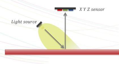
Fig 1 45/0 degree measurement principle.
