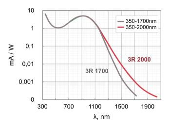
Figure 3. Spectral sensitivity for SM-3R series IR viewers
