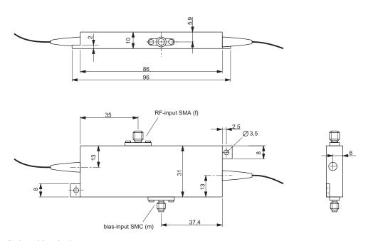
Dimensions amplitude modulator (mm)
