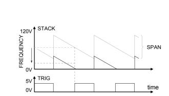
**Figure A.2:** STACK output voltage and trigger pulse, when FREQUENCY is set near the midpoint (upper) or moved closer to  $0\,V$  (lower), where the output voltage exceeds the maximum range.
