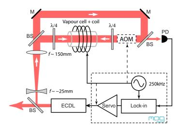
**Figure 3.5:** Schematic setup for AC locking to an atomic transition. PD is the DLC photodetector. BS beamsplitter, M mirror,  $\lambda/4$  retarder. Beam expanding lenses increase signal power without power broadening.
