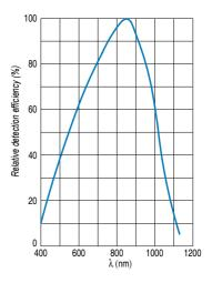
Figure F.3: Photodiode spectral response, standard filtered and unfiltered.
