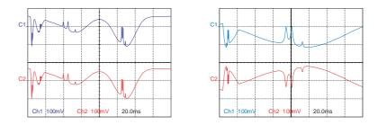
**Figure 3.4:** Examples of spectra for DC locking, for wide and narrow spans (upper traces) and error signals (lower traces).
