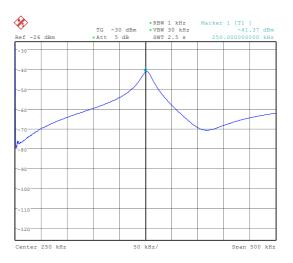
**Figure D.3:** Coil response acquired using a spectrum analyser with tracking generator. The response shows a strong resonance near 250 kHz.
