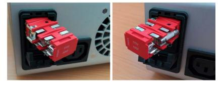
Figure K.5: Bridge (left) and fuse (right) for 115 V.
