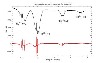
**Figure 3.2:** A saturated absorption spectrum of rubidium using a standard uncoated laser diode and low diffraction efficiency grating in Littrow configuration (upper trace). The lower trace shows the AC-modulation error signal (see §3.5).
