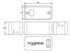
**Figure F.2:** M4 mounting holes are marked with a dimple; others are 8-32. Single channel photodiode 1, differential signal 1 - 2.
