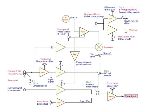
Figure H.1: Overview of error signal.
