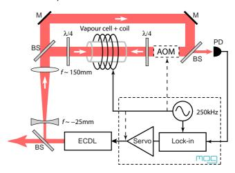
**Figure 1.5:** Setup for AC locking to an atomic transition. PD DLC photodetector, BS beamsplitter, M mirror,  $\lambda/4$  quarter-wave retarder. See also Figs. 3.5, 3.6.
