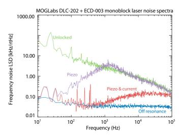
**Figure 4.1:** Error signal spectra, with laser unlocked, locked with SLOW (piezo) feedback only, and with SLOW and FAST (piezo+current) feedback. The off-resonance spectrum provides information on the effective noise floor.
