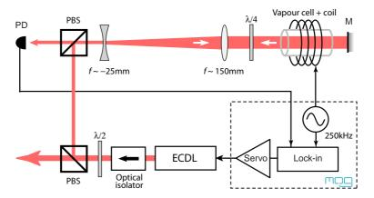
**Figure 3.6:** Schematic setup for a more compact and more easily aligned saturated absorption arrangement. PD is the DLC photodetector. PBS polarising beamsplitter, M mirror,  $\lambda/4$  and  $\lambda/2$  retarders. Beam expanding lenses increase the signal power while minimising saturation broadening.
