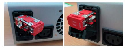
**Figure K.4:** Bridge (left) and fuse (right) for 230 V. Swap the bridge and fuse when changing voltage, so that the fuse remains on the right-hand side (see below).
