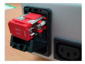
**Figure K.1:** Fuse catridge, showing fuse placement for operation at 230 Vac.
