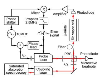
**Figure E.2:** High bandwidth locking based on FM sideband demodulation [11, 6]. The probe laser is locked with high bandwidth, relative to the coupling laser, using electromagnetically induced transparency as a dispersive reference.
