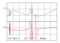
**Figure 3.7:** Examples of spectra for AC locking, for wide and narrow spans (upper traces), with error signals (lower traces).
