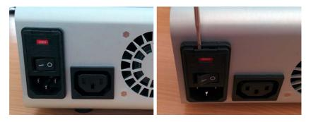
**Figure K.2:** To change fuse or voltage, open the fuse cartridge cover with a screwdriver inserted into a small slot at the top of the cover, just above the red voltage indicator.
