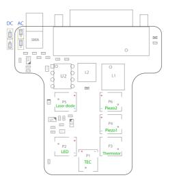
**Figure G.3:** B1047 enhanced laser head board. Jumpers at top left can be configured for AC or DC coupling. Modulation input via SMA connector, sensitivity 2.5 mA/V. The B1240 is almost identical but has an additional jumper for direct or differential ground coupling adjacent to U2.
