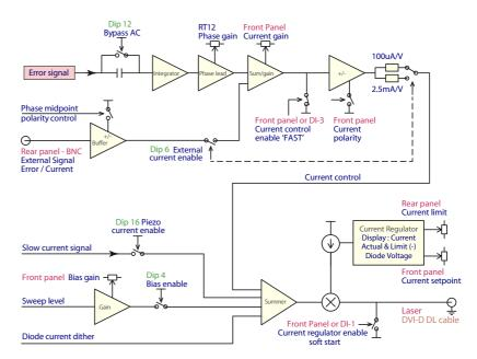
Figure H.3: Overview of fast feedback and diode current signals.
