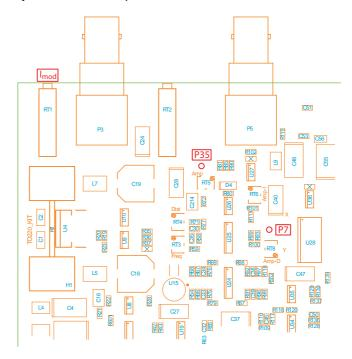
**Figure B.1:** 250 kHz oscillator trimpots and testpoints.
