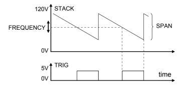
**Figure 1.2:** Stack (or current bias) output and trigger pulse, when scanning. Note that the ramp slope can be inverted. Details of the ramp behaviour are described in section A.2.
