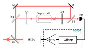
**Figure 3.3:** Schematic setup for DC locking to an atomic transition. PD is the DLC photodetector. BS beamsplitter, M mirror,  $\lambda/4$  retarder.
