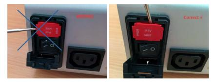
**Figure K.3:** To extract the fuse cartridge, insert a screwdriver into a recess at the *top* of the cartridge.
