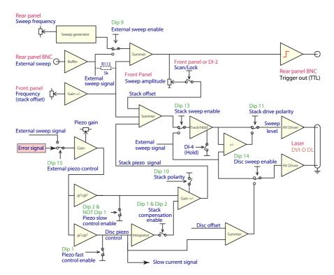
**Figure H.2:** Overview of slow feedback and piezo signals. Note that resistor R113 is not installed by default.
