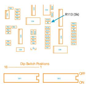
**Figure 3.8:** R113 is connected so that signals on the SWEEP input always affect the piezo. Remove if using external sweep, or add if using external *control* signal to drive the piezo.
