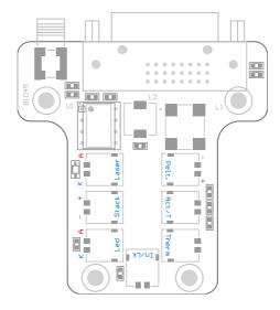
**Figure G.2:** MOGLabs B1045 laser head board showing connectors for laser diode, piezo actuator, temperature sensors, TEC and head enclosure interlock.
